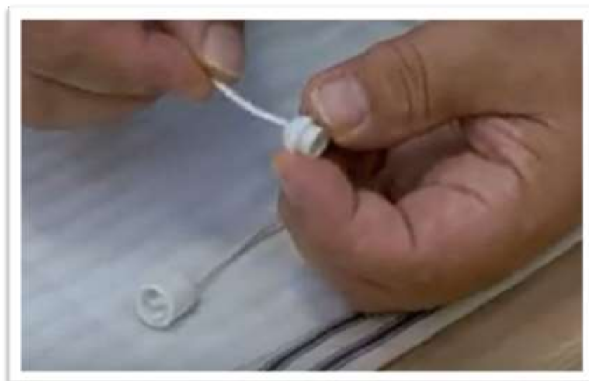
Figure 27: Installing a Cord Condenser
