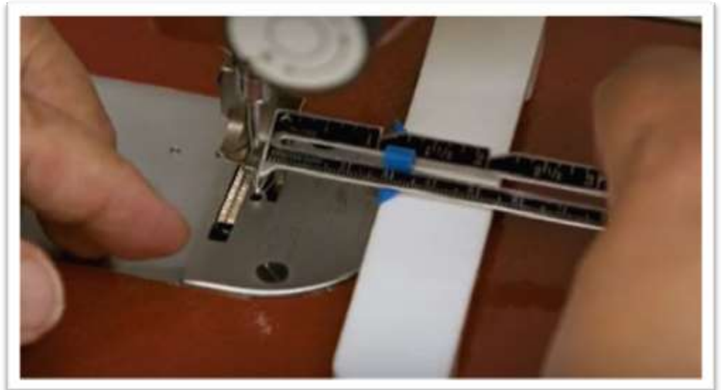
Figure 15: Measuring for the Slat Pocket Seam
